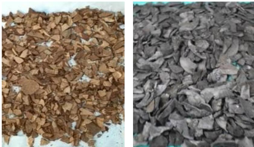
Figure 1. (a) Coconut shell before carbonization and (b) Coconut shell after carbonization
