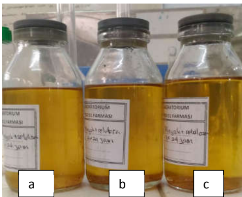
Figure 3. Used Cooking Oil after Immersion by Using Nanocellulose (a) 1 x 24 hours (b) 2 x 24 hours (c) 3 x 24 hours
