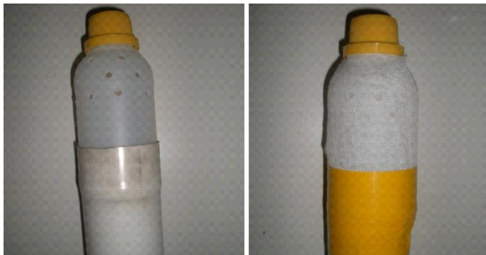
Figure 2. Peeping bottle designed to collect porewater sulfide. The upper side of the bottle had holes around it, covered with a soft net, and was connected to a PVC pipe
